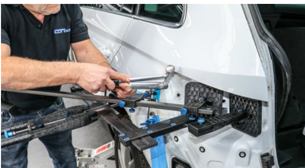
Insert with double foot when pressing
