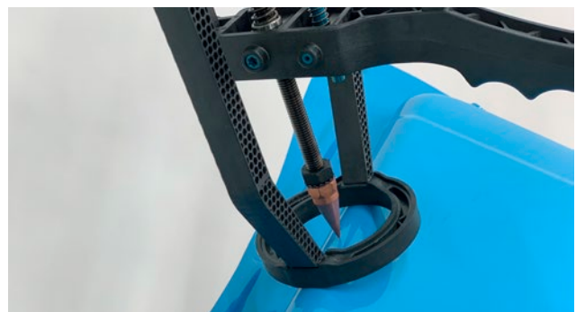
Correct The pressure point of the outriggers must be diagonal to the edge.
