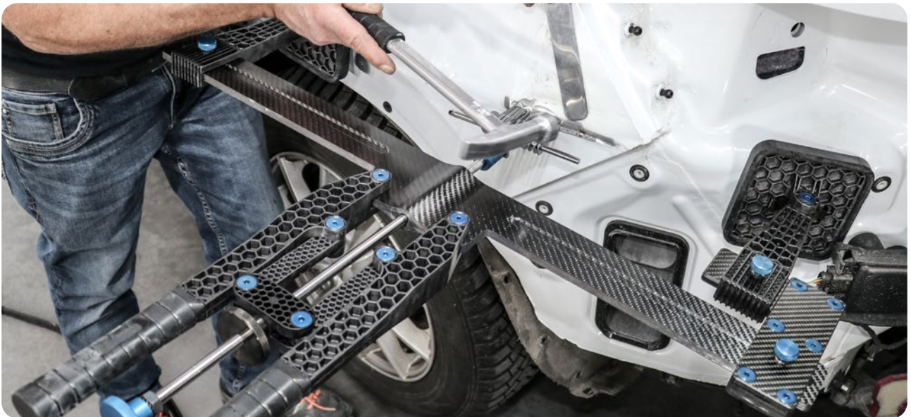
The StrongTool with the optional support in the engaged state
